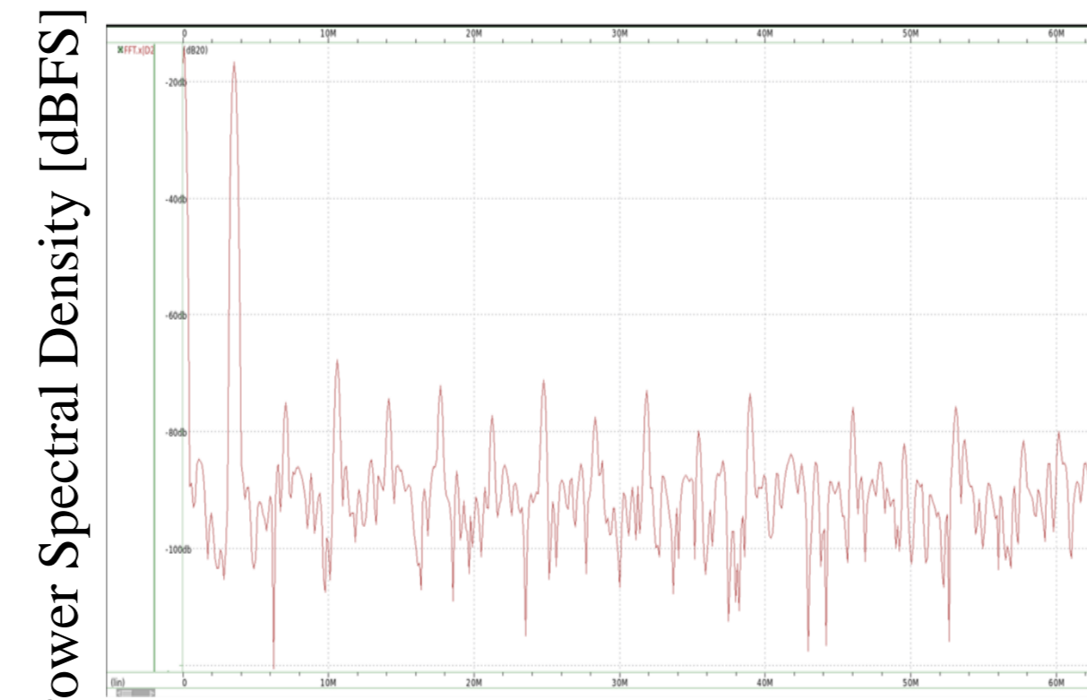
Fig. 8. Pre-simulation 1024-point FFT spectrum at 125 MS/s (@TT,0.8V,25°C)
